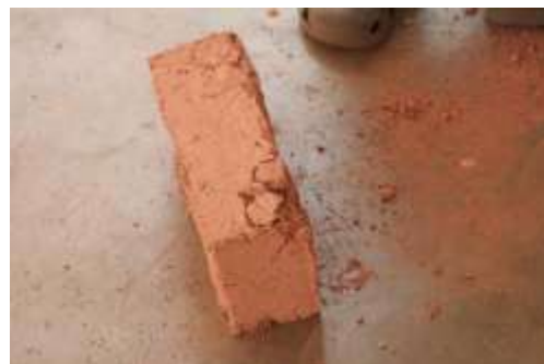
Uneven edges and poor quality brick
