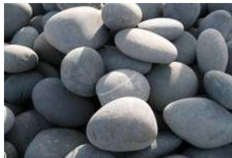
Poorly shaped stones, rounded edges
