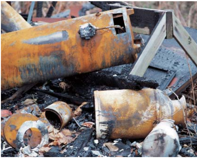
Water heater burned in residential fire caused by a gas leak.
