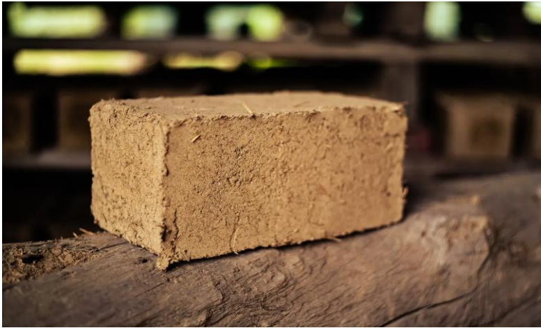
Fig. 7.6.2.1. Soil stabilized bricks
