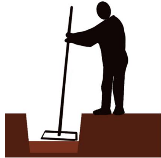
Fig. 6.1.6. ground hardened by a rammer
