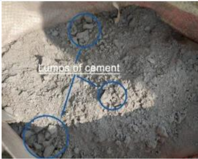
Fig 7.1.2. Lumps of Cement due to moisture
