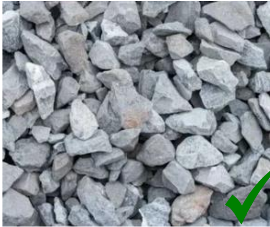
Fig 7.3.1. Sharp edged aggregate vs round aggregate
