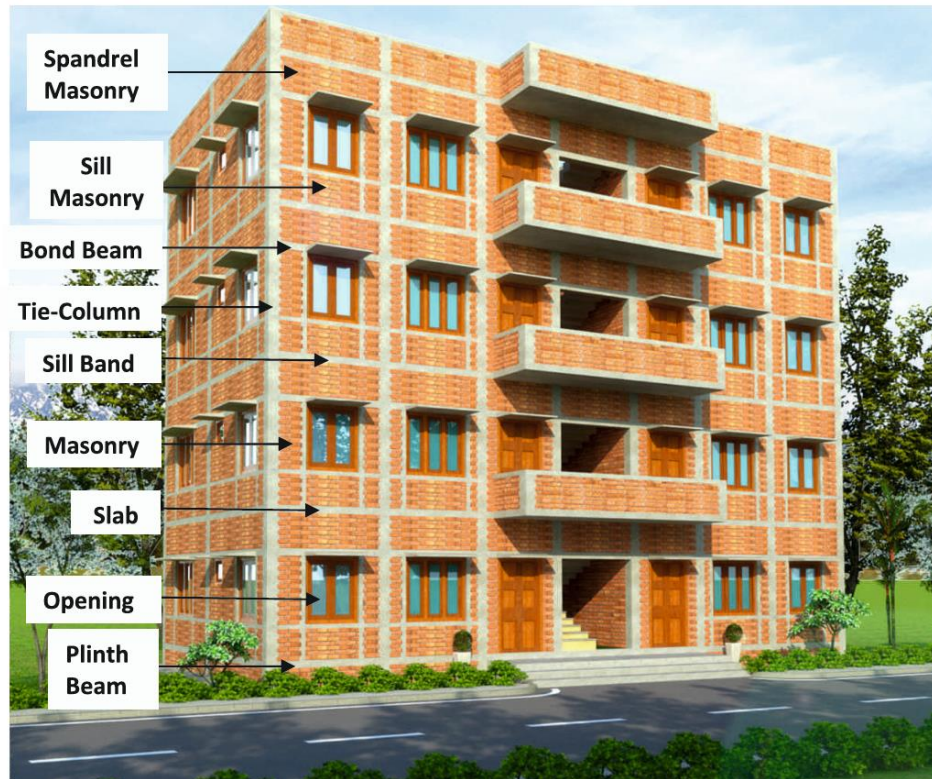
Fig 6.3.1. Components of confined masonry
