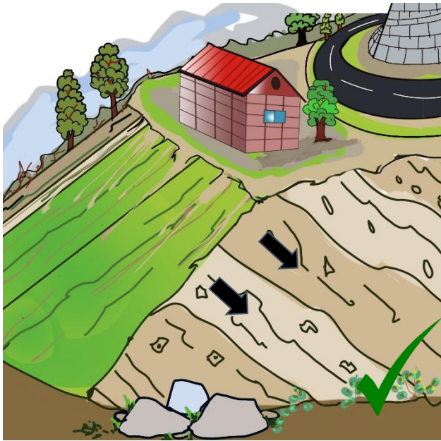
a) Rock slope into the hill
