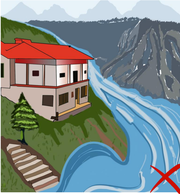
Fig 3.2.3.1 Proximity to Water Body
