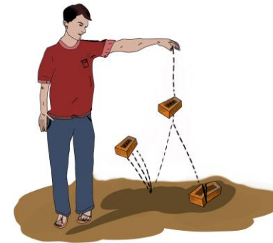
Fig. 7.6.1.4. Strength testing for brick
