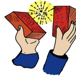
Fig. 7.6.1.2. Metallic sound of bricks
