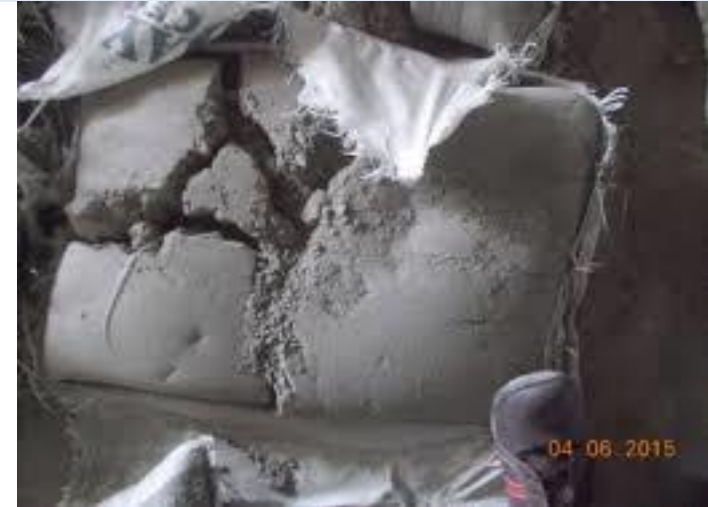
Fig 7.1.3 Cement bags after 3 months
