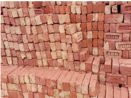
Fig. 7.6.1.3. Dry bricks to not be used
