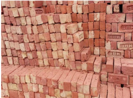
Fig. 7.6.1.3. Dry bricks to not be used
