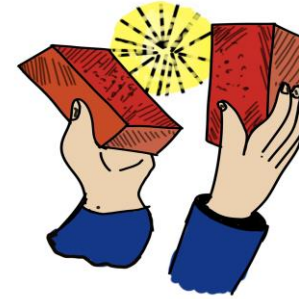
Fig. 7.6.1.2. Metallic sound of bricks
