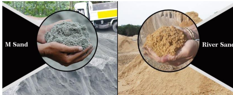
Fig 7.2.1. Identification of different types of sand
