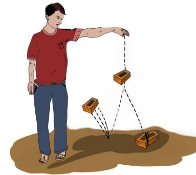
Fig. 7.6.1.4. Strength testing for brick
