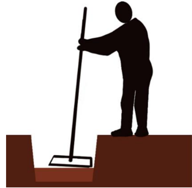
Fig. 6.1.6. ground hardened by a rammer
