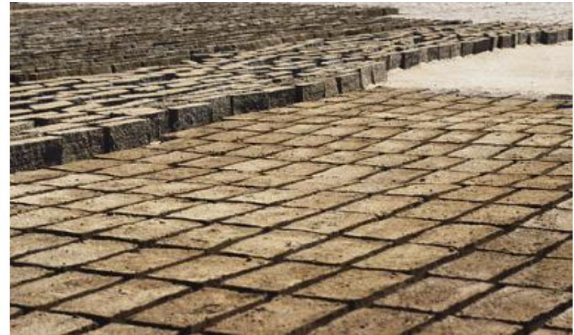
Fig. 7.6.2.2. Sun dried bricks drying
