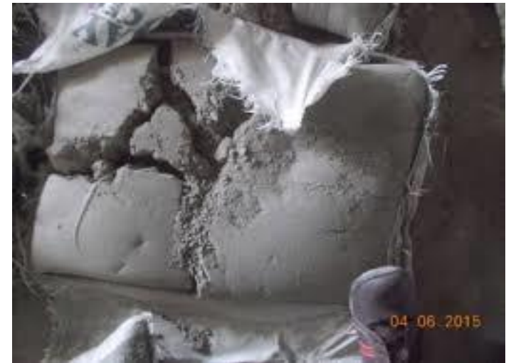
Fig 7.1.3 Cement bags after 3 months
