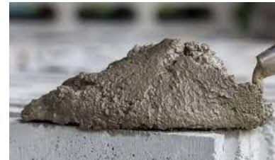
Cement mortar consistency
