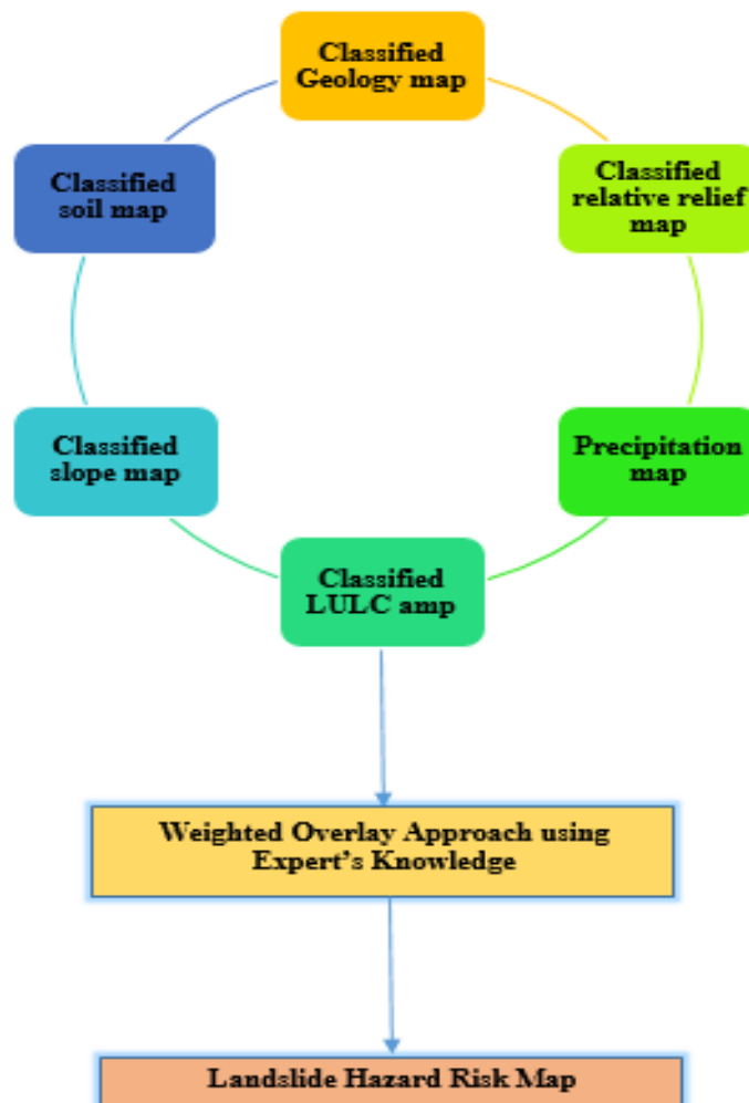
Figure 2: Flowchart for Hazard Mapping
