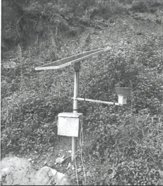
Our Contribution: Low – cost Landslide Monitoring System
