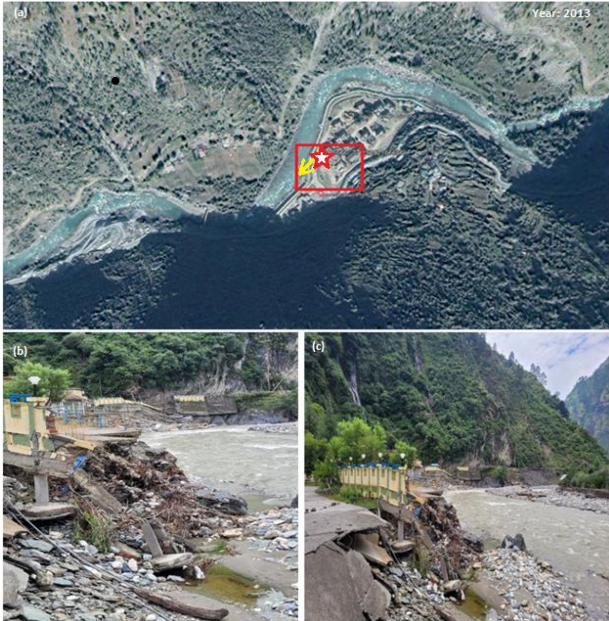
Fig. 13: Extensive damage to road infrastructure and collapse of retaining walls near NHPC residence at Spangani village caused by severe flash flooding. Major landslide visible on the opposite riverbank covering a span of around 100 meters.
