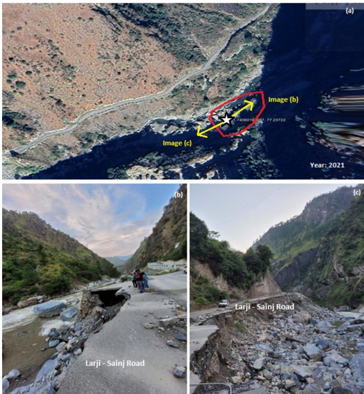
Fig. 23. In Bihali village, the paved road stretching approximately 300 meters constructed along the riverbank has been completely washed away due to flash floods eroding away the banks.
